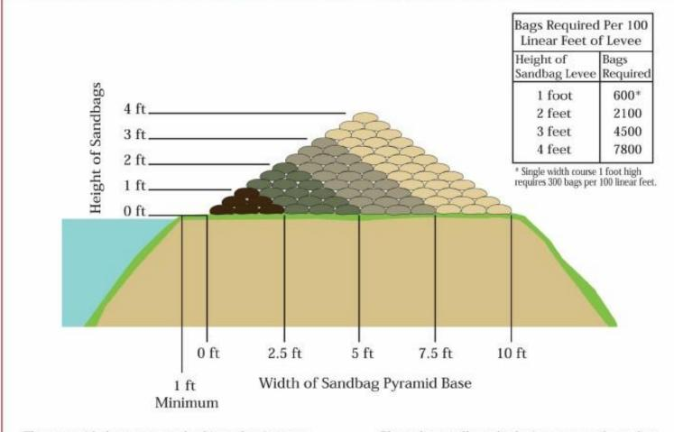
The pyramid placement method issued to increase the height of sandbag protection.
